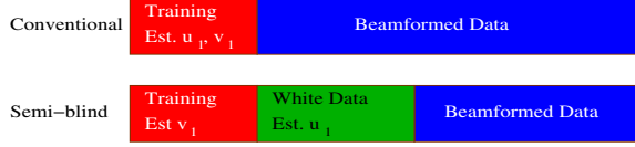
Fig. 1. Comparison of the transmission scheme for conventional least-squares (CLSE) and closed-form semi-blind (CFSB) estimation.
