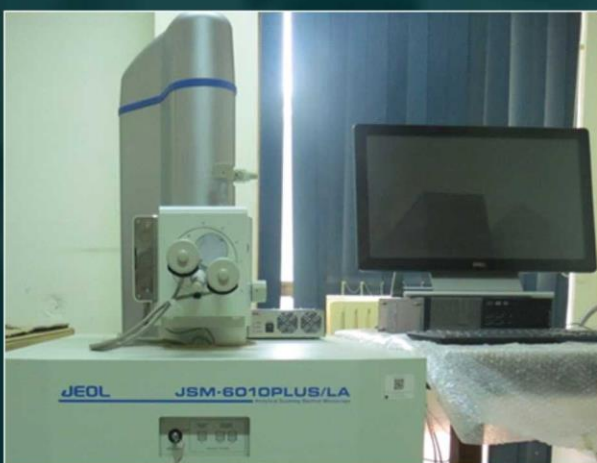
Scanning Electron Microscope EM, JSM-6010PLUS/LA, JEOL Asia Pte
