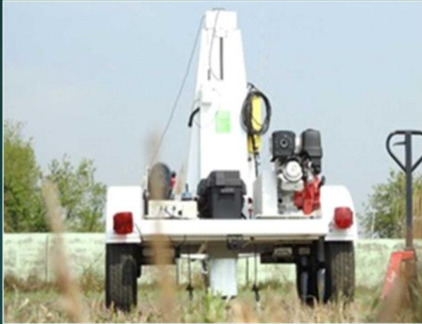
ESS1000 WITH 950-1000 Pound hammer (seismic energy source)
