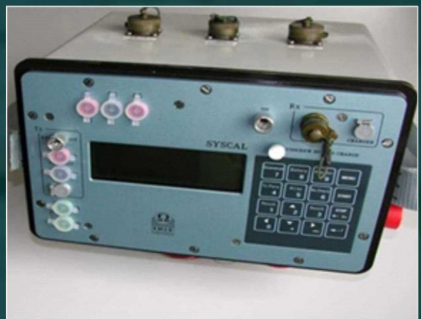
SYSCAL Junior R1 Plus Switch-72 Resistivity meter, SYSCAL Junior R1 Plus Switch, Iris Instrument, France
